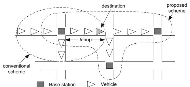
**Fig. 2** The conventional Multihop Cell scheme vs. the proposed Roadside Multihop Cell scheme
