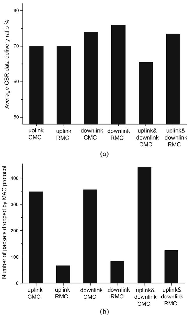
**Fig. 11** Study of impact of mobility management overhead. **a** Comparison of average CBR traffic data delivery ratio under different scenarios. **b** Comparison of number of packets drop by MAC protocol
