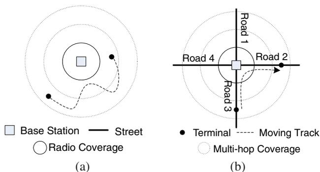
**Fig. 3** Comparison of mobile nodes in general networks and vehicular networks. **a** General mobile nodes move freely in two dimensions. **b** Vehicles move along the roads
