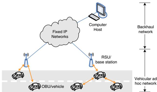
**Fig. 1** The architecture of a vehicular network
