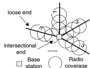
**Definition 2** A Roadside Multihop Cell is constructed by adjacent Directional Multihop Cells that have a common loose end.
