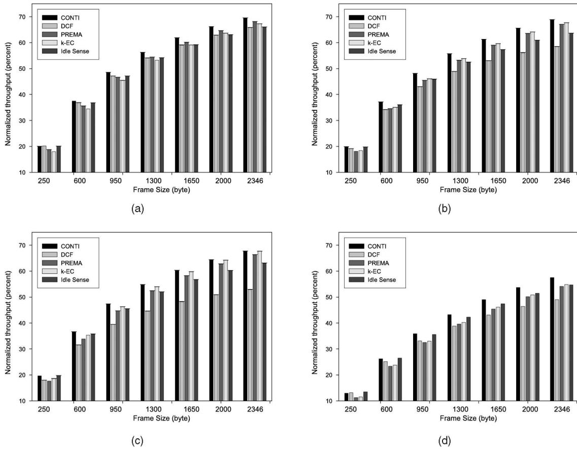
Fig. 5. Throughput with IEEE 802.11b&g. (a) Throughput of five stations with IEEE 802.11b. (b) Throughput of 20 stations with IEEE 802.11b. (c) Throughput of 50 stations with IEEE 802.11b. (d) Throughput of 20 stations with IEEE 802.11g.
