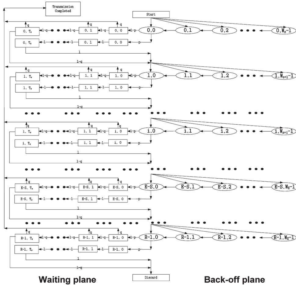
Fig. 2. MC model for contention resolution.
