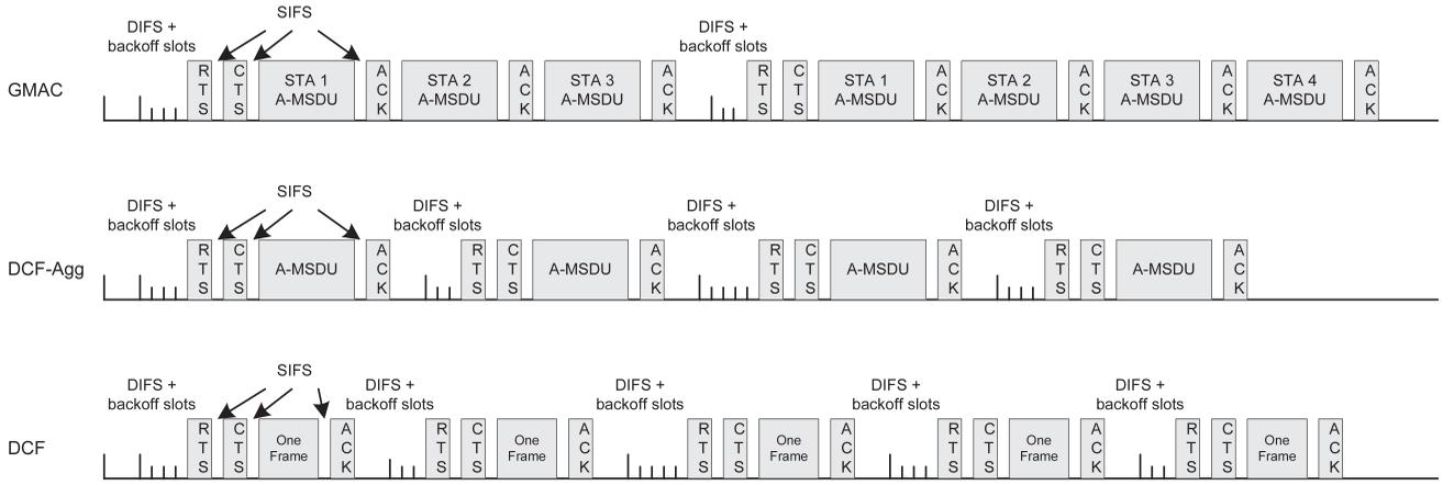
Fig. 4. Transmission of GMAC, DCF-Agg, and DCF.
