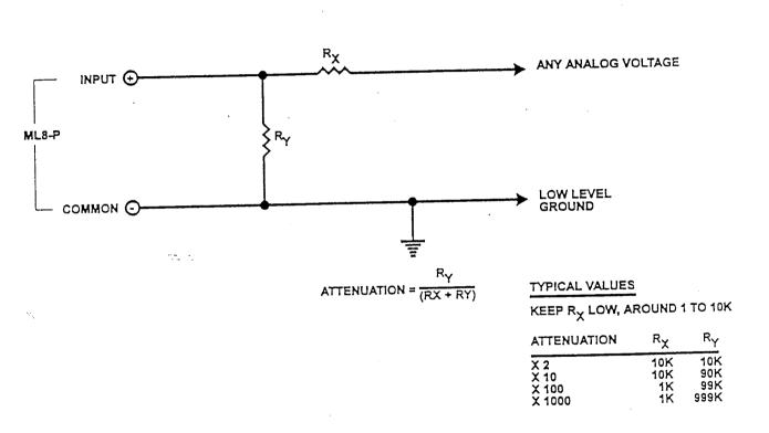
Figure 2 Voltage Attenuation for greater than 5VDC
