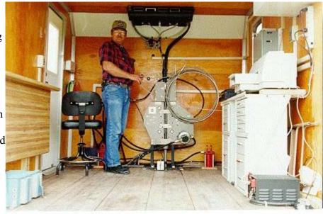
quickly perform on-site soil characterization tests. This system is especially effective in satisfying soil investigation needs of highway engineering.
