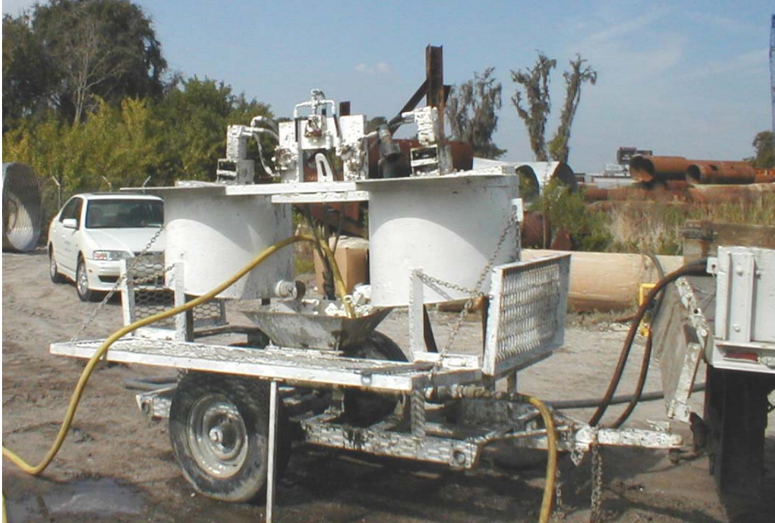
Figure 8. Trailer Mounted Grout Mixing and Pumping System.
