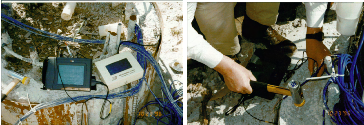
Figure 20 Equipment used for sonic echo test (left), impact hammer struck on shaft head (right). (Courtesy of Applied Foundation Testing, Inc.)
