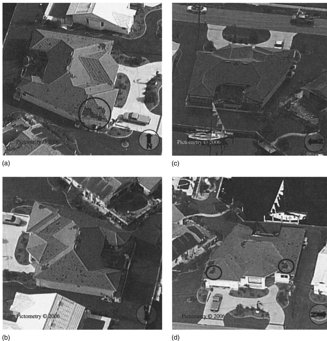
Fig. 3. Example neighborhood oblique image. Four views allow for damage on all sides to be clearly seen and estimated: (a) south; (b) north; (c) west; and (d) east views of a damaged house (Reprinted with permission, Pictometry International Corp. 2006).
