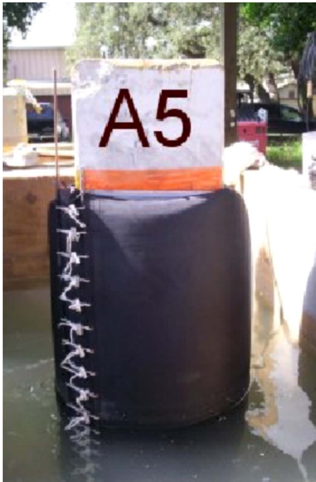
Fig. 9. Pressure bag applied to prepreg system
