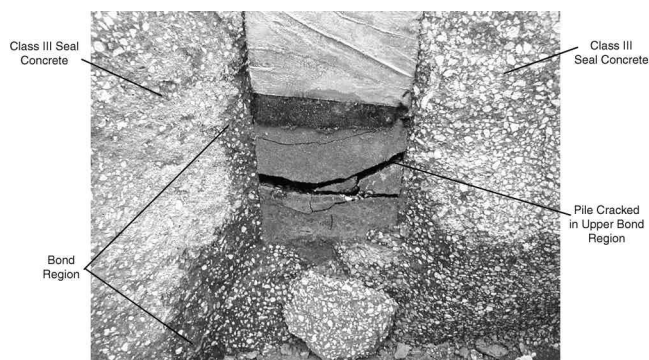
Fig. 5—Postmortem profile view of pilot study specimen during dismantling.
