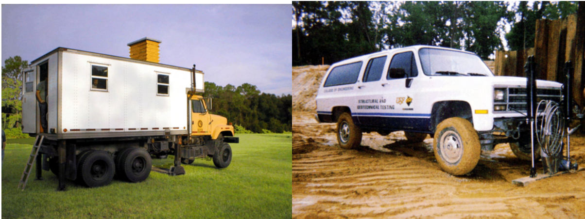
Figure 15 Standard 20 ton cone truck (left); 4 ton mini-cone vehicle (right).
