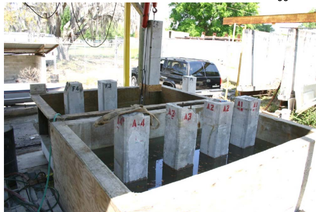
Fig. 5. View of partially submerged full-size test piles
