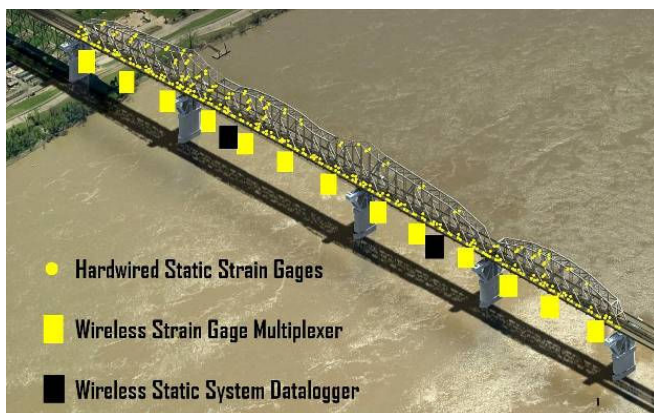
Fig. 12. Placement of gages
