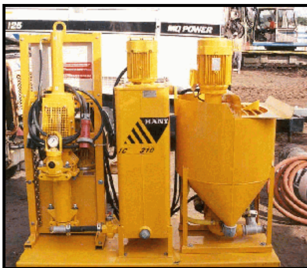
Figure 8. Three part grout plant.
