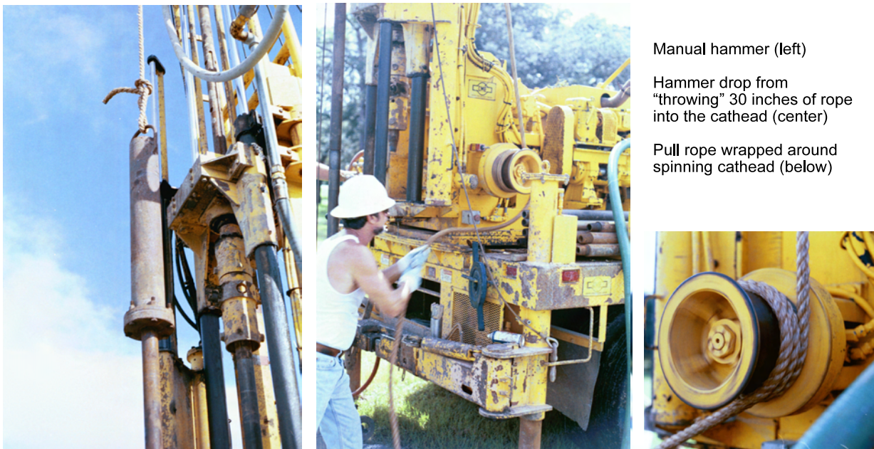
Figure 5 Manual hammer SPT apparatus.
