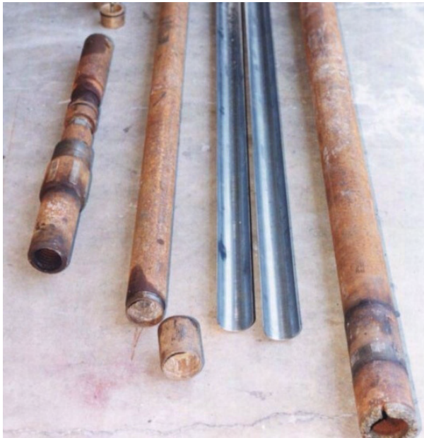
Figure 9 Triple tube core barrel components.
