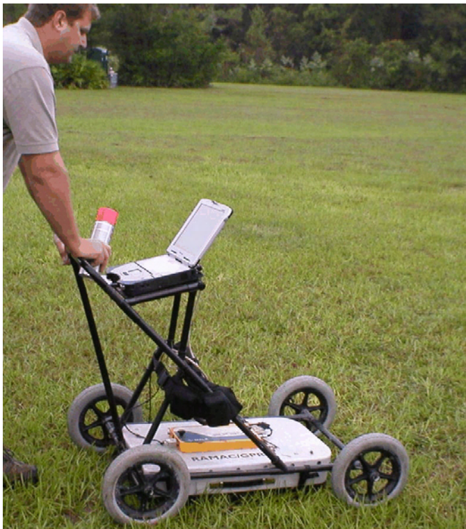
Figure 1 GPR field device (Courtesy of Universal Engineering, Inc.).
