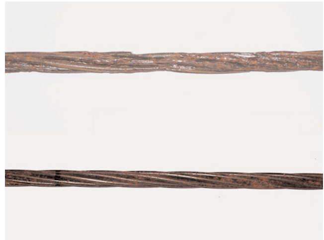
FIGURE 2 Retrieved strands after 38 months of exposure to outdoor simulated tidal cycles in 3% saltwater: unwrapped (top) and FRP wrapped (bottom).
