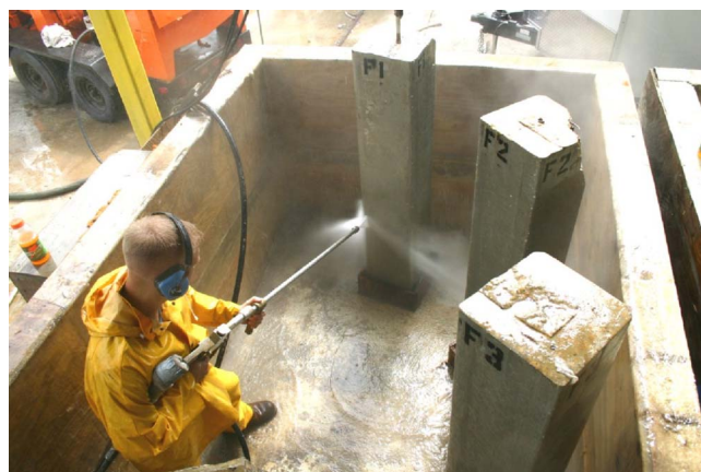
Fig. 6. Pressure washing test piles with 68.9 MPa water pressure
