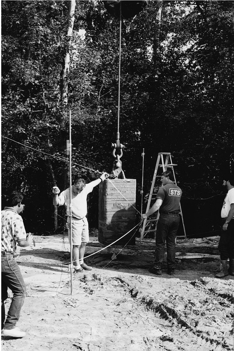
Fig. 5. Weight positioned between poles with mounted laser photocells.
