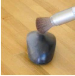
If the object is reflective or transparent for a more accurate scan of the surface it will be better to use a powder prior to scanning. Align the object on the scanning platform once it prepared.
