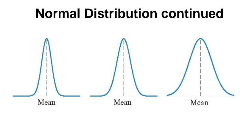
The shape of the normal distribution depends on the mean and the standard deviation. These three graphs have the same mean but different standard deviations. As the standard deviation increases, the distribution becomes more spread out.
