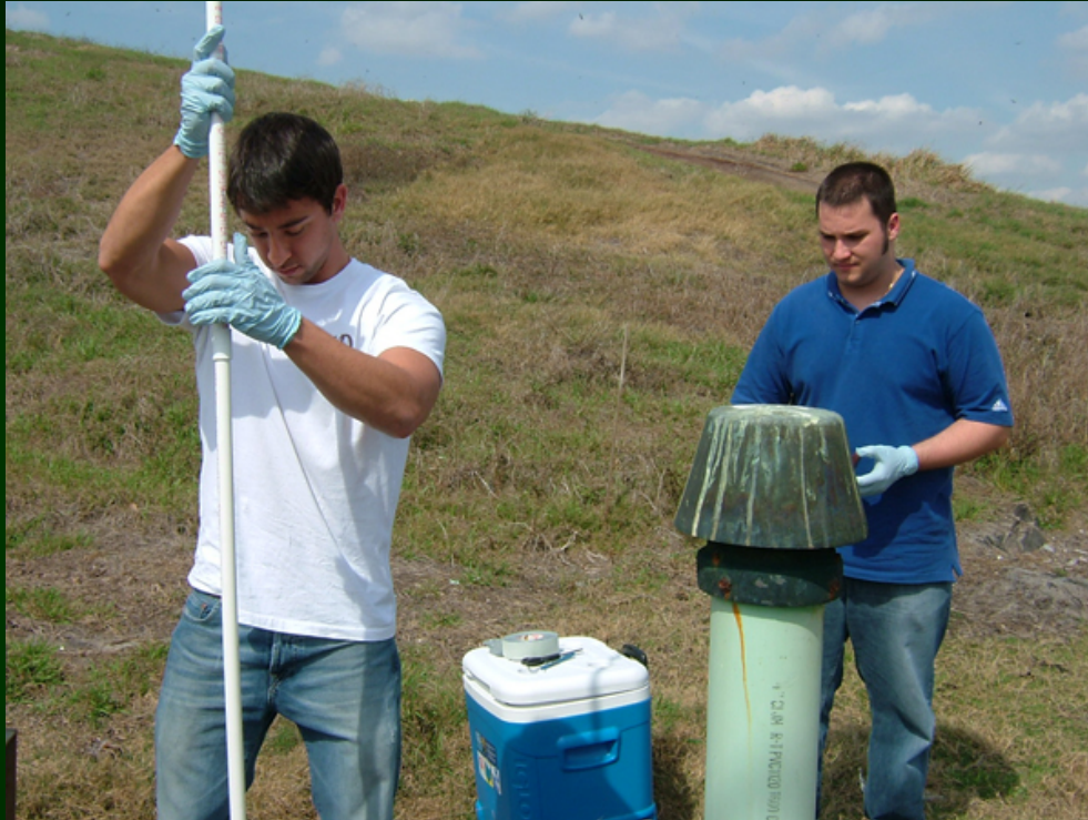
Ryan Locicero (graduating senior) and Austin Roe (first year honor's student) taking a sample of phase II leachate at the North Central Landfill in Polk County
