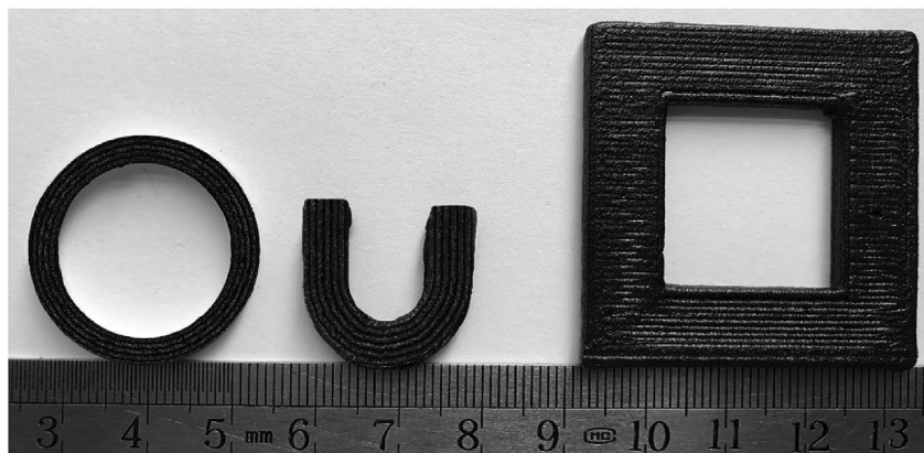
Fig. 12. Complex-shaped NdFeB bonded magnets with 20 wt.% SrFe 12 O 19 prepared by 3D printing.
