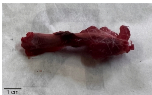
Figure 4. Macro-photograph of the femur of a laboratory rat implanted with NiTi with 0.5 at. % Ag in the distal part 75 days after implantation.
