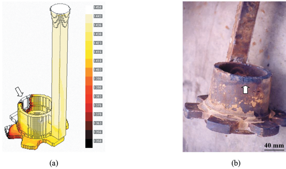
Figure 5. Mould filling simulation showing the chilled melt front (the units are °C) (a) and the corresponding defect of a lost form hub casting (b). The material is ductile iron 65–45–12 and the pouring temperature is 1450°C.
