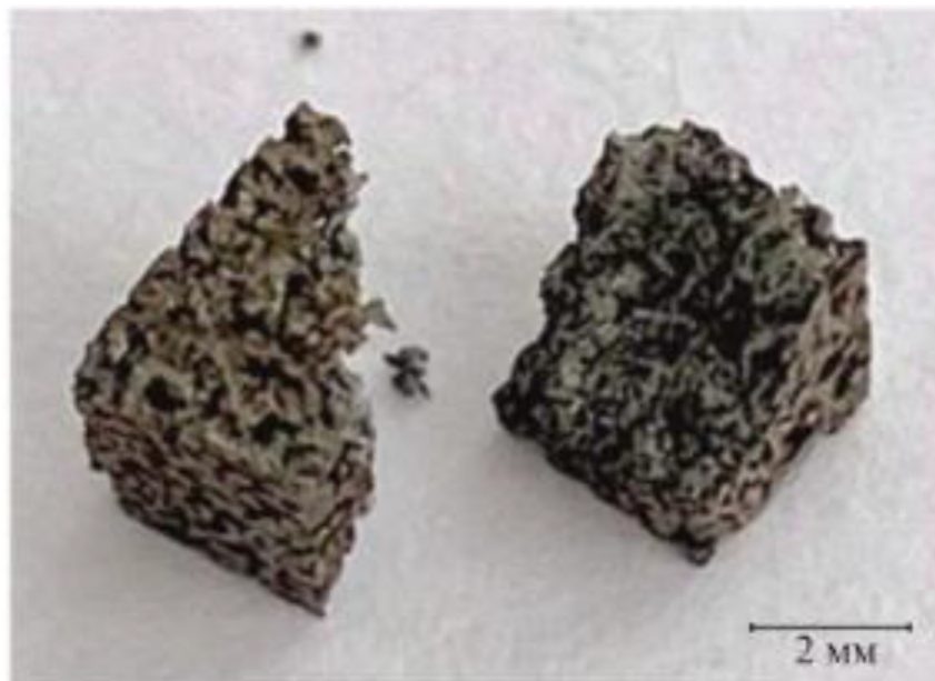
Fig. 7 – Porous SHS-NiTi sample after compression failure.
