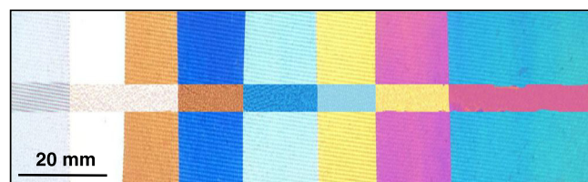
FIGURE 6 Color of eight PVC films package in transmitted polarized light after local heat treatment of the outer layer (band in the center). [Color figure can be viewed at wileyonlinelibrary.com ]
