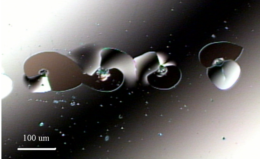
Figure 138. Al film spallation and circumferential cracking (Al 340 nm film on Cu, 1 \mu\text{m} W 100 MPa tensile residual stress).
